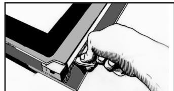
Lever the assembly to detach the frame and the glass.
