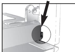
Attach the frame by tightening it with the door. Do not press on the frame alone.
