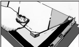
This assembly comprises 2 glass windows, the 1st of which has 2 rubber stops on the 2 front corners.
