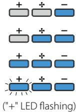
Speed 1<br>Speed 2<br>Speed 3<br>Speed 4<br>("+" LED flashing) |
