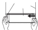
**Installation :** Hold both sides of the bottle shelf with both hands. Install the buckle of the boss side at first. Then push the other side inward slightly, the buckle can be fixed.
